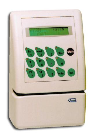
Synel's SY-71X series of intelligent, programmable data collection terminals is designed for cost effective Time & Attendance applications. The terminals are ideal for fast and precise internal data reporting, with both the security of a self-contained unit and the flexibility of a PC-linked system.
